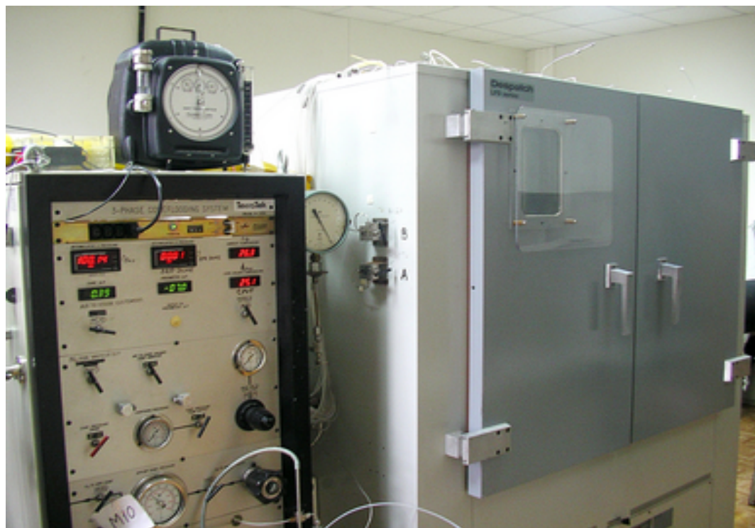
Figure 3 – General view of control cabinet (left) and filtering unit (within thermostatic box, right)
